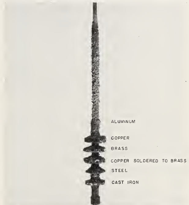
FIGURE 14. Metal test specimens after 537 hours in magnesium chloride antifreeze.
