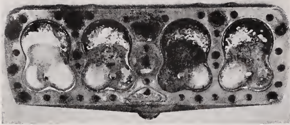
FIGURE 7. Aluminum cylinder head after 734-hours operation on magnesium chloride antifreeze.
