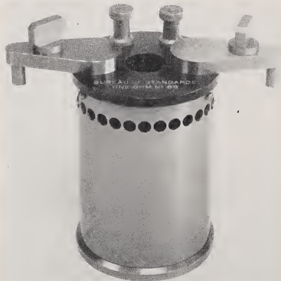
FIGURE 4. Double-walled standard resistor.
