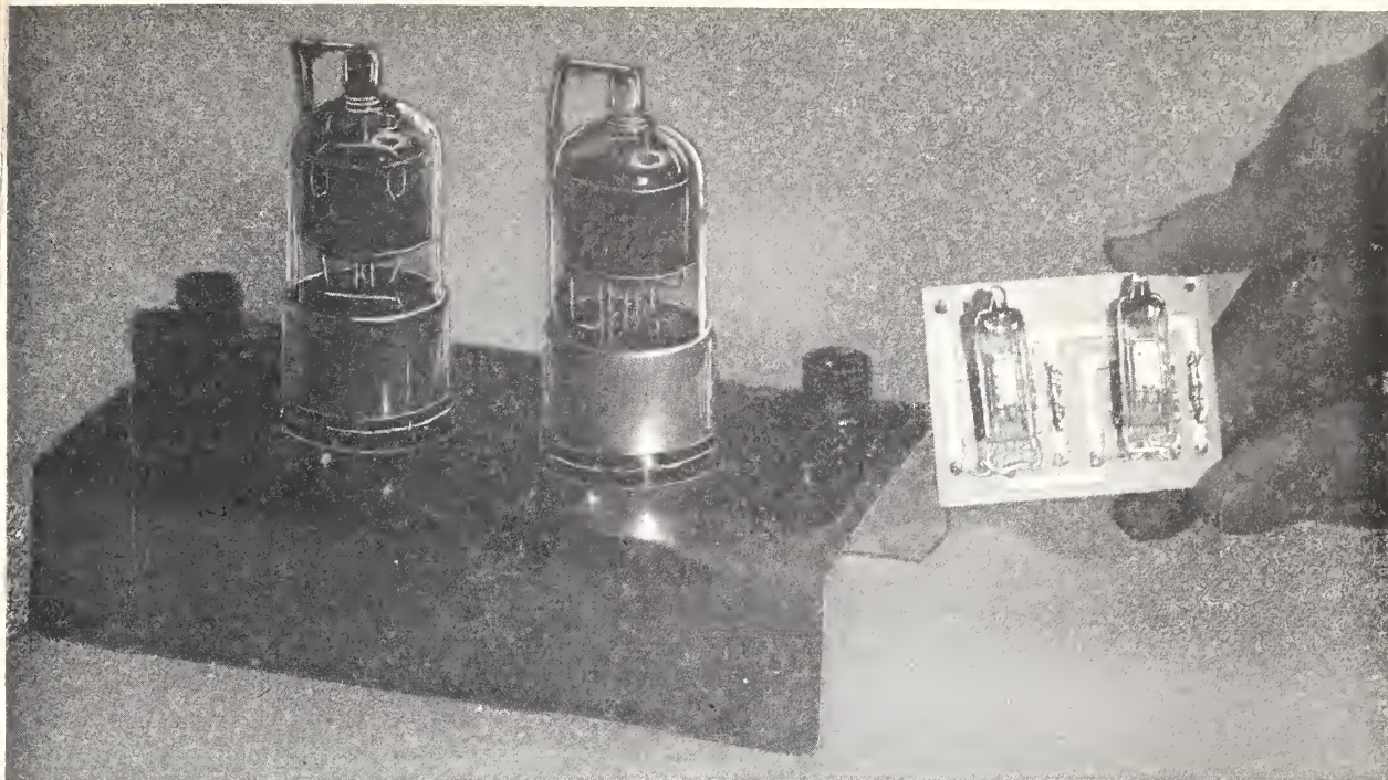
FIGURE 2. Comparison of two-stage voltage amplifier printed on ceramic plate (right) with equivalent amplifier constructed according to present day radio practice (left).
