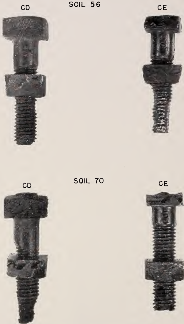
FIGURE 10.—Charcoal cast iron CD, and steel CE, bolts exposed to both soils 56 and 70 for approximately 2 years each.
