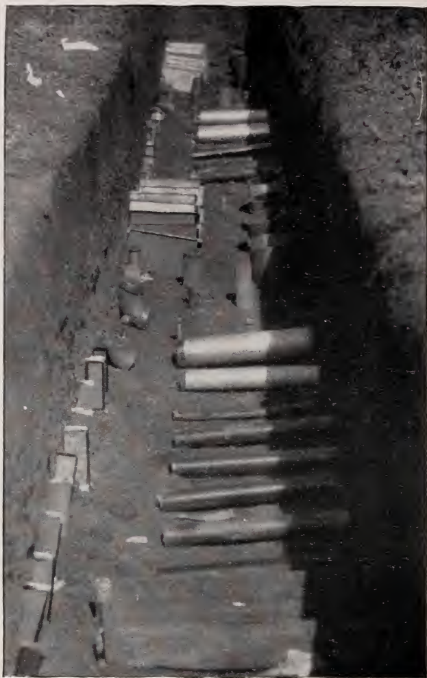
FIGURE 5.— Arrangement of specimens buried in 1924
