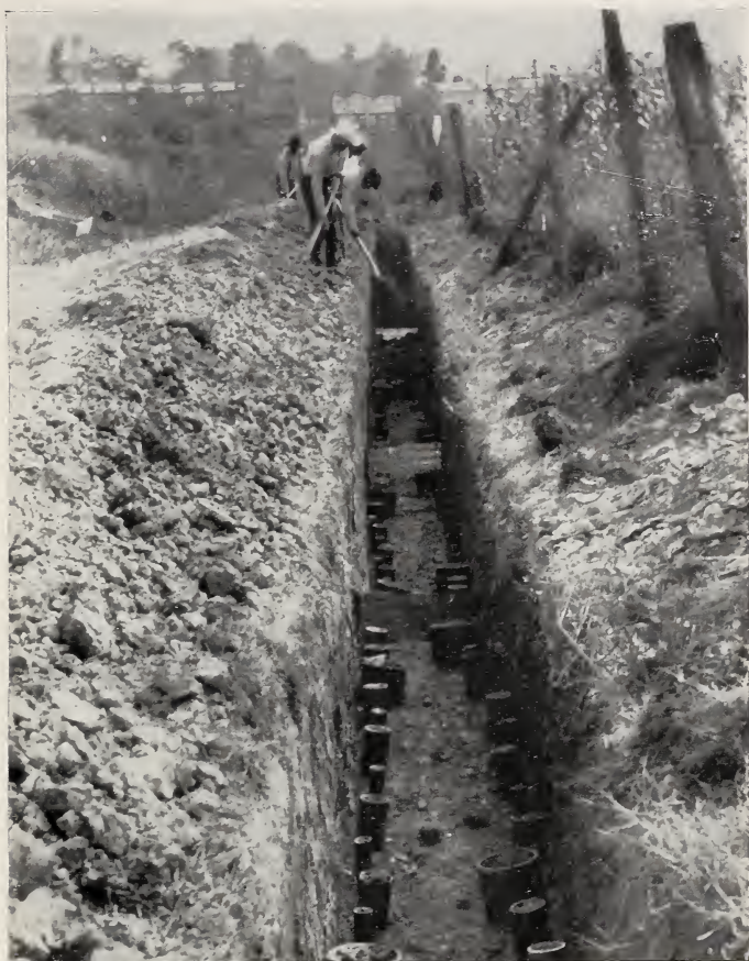
FIGURE 4.—Burial of soil corrosion specimens near Alexandria, Va., in 1922.
