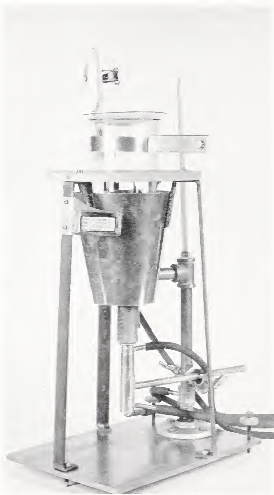
FIGURE 95.—Stove assembly with the burner arrangement illustrated in Figure 5. The boiling-vessel assembly is in position for the carrying out of a candy test.
