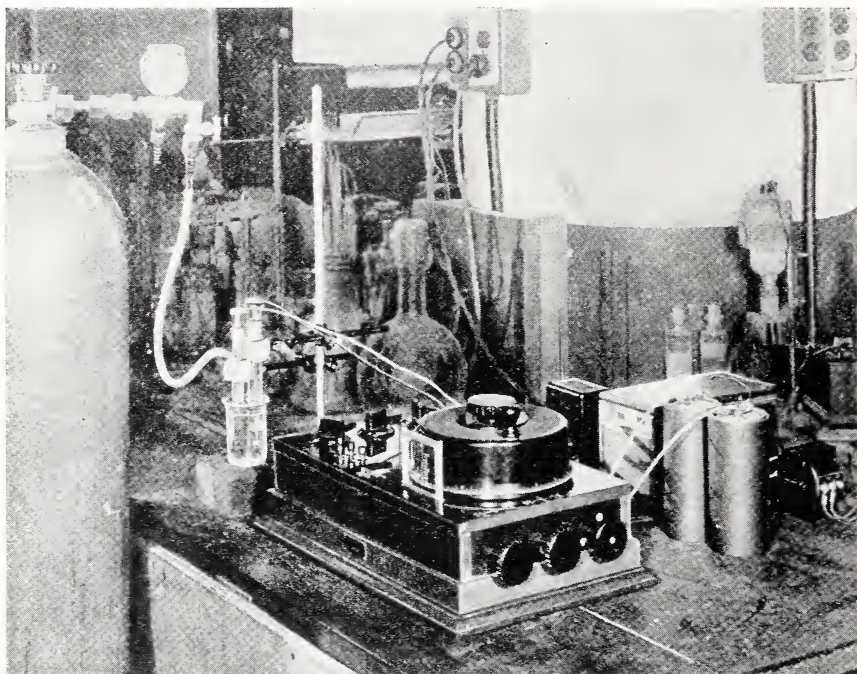
FIGURE 54.—Leeds & Northrup type K potentiometer with hydrogen-gas electrode, calomel electrode, etc.
