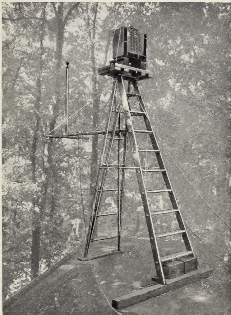
FIGURE 21.— Experimental arrangement for outdoor testing of loudspeakers.
