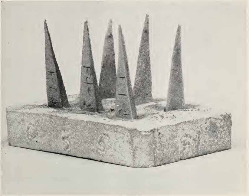
FIGURE 1.—Arrangement of specimens for determination of deformation temperatures.
