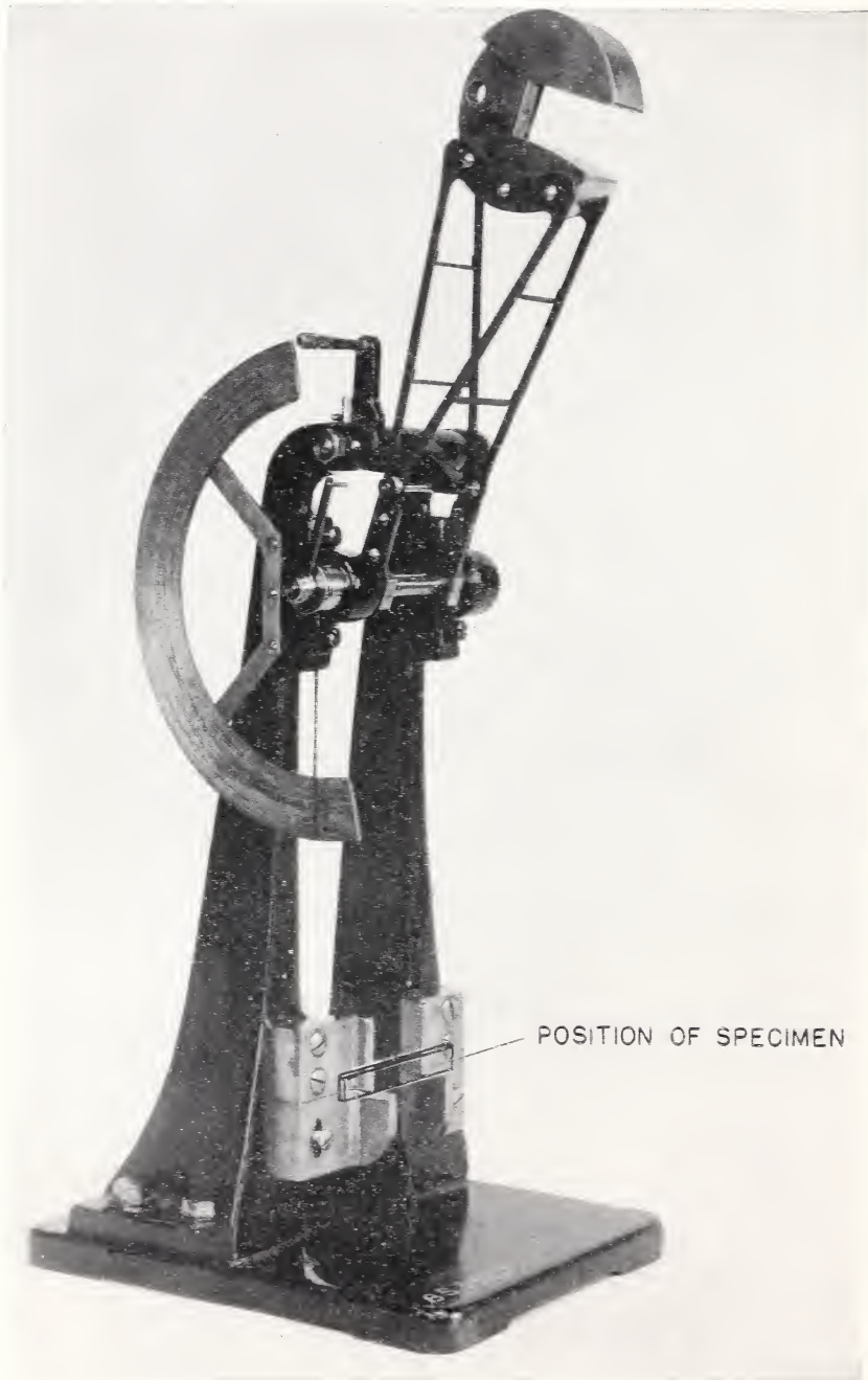
FIGURE 90.—Charpy-type impact machine. One-third actual size
