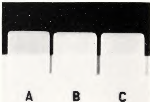
FIGURE 55.—Alabaster glass standards used in determining opacity of silicate cements photographed on a black-and-white background.
