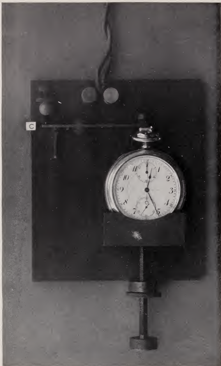
FIGURE 4.— Special key used in the testing of stop watches.
