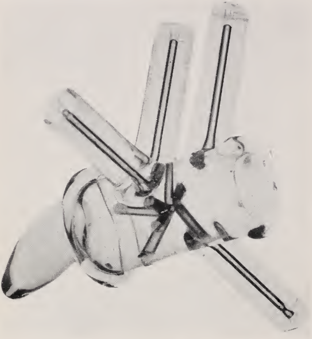
FIGURE 5.— Stopcock which functions both as a tee cock of a gas distributor and a cock at the top of a bubbling-type absorption pipette.
