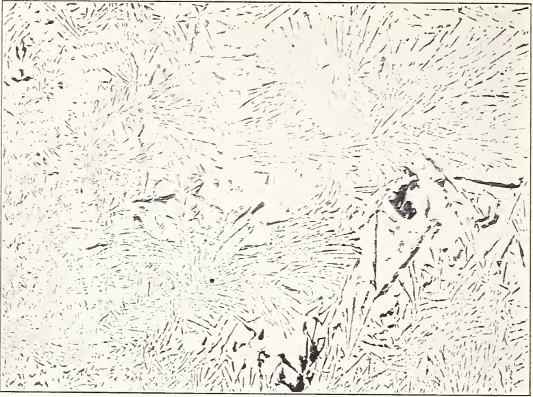
FIG. 65.— Structure of 13 per cent silicon alloy, unmodified. \times 100 —unetched
