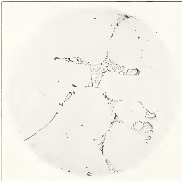
FIG. 3.— Structure of ingot aluminum. \times 500 Etched in 1 per cent HF to which a few drops of \text{HNO}_3 were added. Illustrates the "Chinese script" formation of the iron constituent appearing in ingot aluminum of 99.14 per cent purity. Only one iron constituent appears in this specimen. (Aluminum Company of America)
