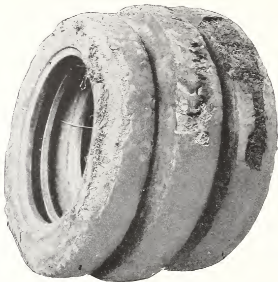
FIG. 11.— Tread abrasion of pneumatic tires due to rough roads
