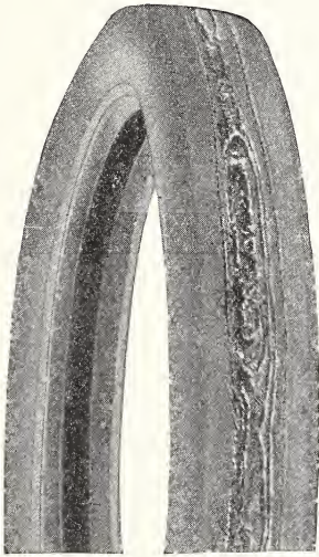
FIG. 9.—Tread wear caused by the misalignment of wheels
