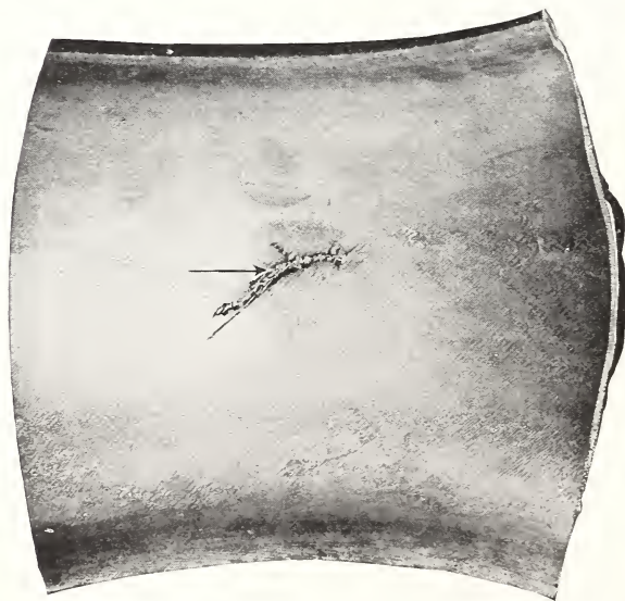
FIG. 17.— Tire injury caused by a sharp blow
