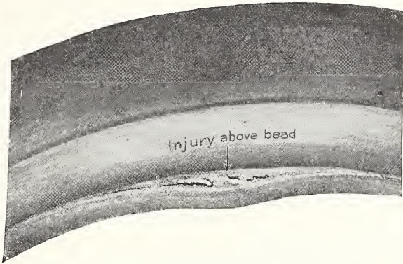
FIG. 4.—Clincher tire injured by bent rim
