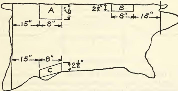
Fig. 1.—Diagram of side showing locations and sizes of samples
