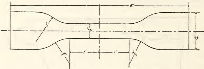
FIG. 2.—Specimen for strength and elongation
