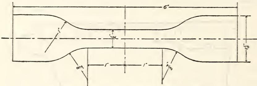
FIG. 2.—*Specimen for strength and elongation*
