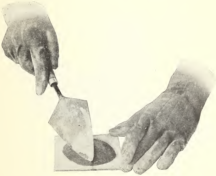
Fig. 4.—Correct Method of Molding Cement Pat
