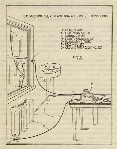
metallic conductor to the ground. If there are no water pipes or radiators in the room in which the receiving set is located, the wire should be run out of doors and connected to a special ground below the window. The ground for the lightning switch should not be used for this purpose. It is essential that for the best
