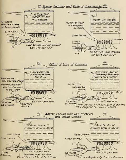
If the present natural gas burners now in use were operated with a fixed orifice and a pressure of about 2.5 inches service complaints would be fewer. Improved burners require only 1.0 inch of gas pressure to inject the air into the burner.
