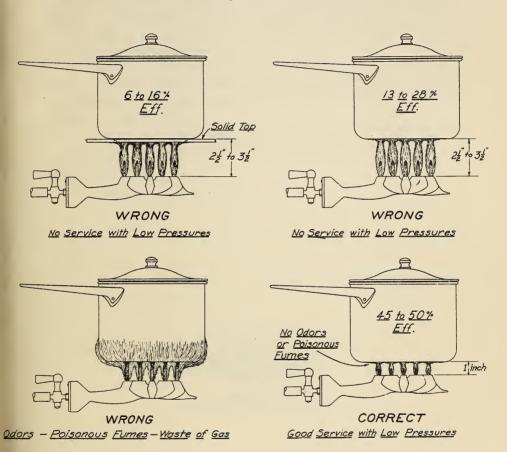
If the solid tops of stoves are removed and replaced by grids, the burners raised, and all domestic appliances operated correctly, at least \$1,000,000 worth of natural qas would be saved daily.
