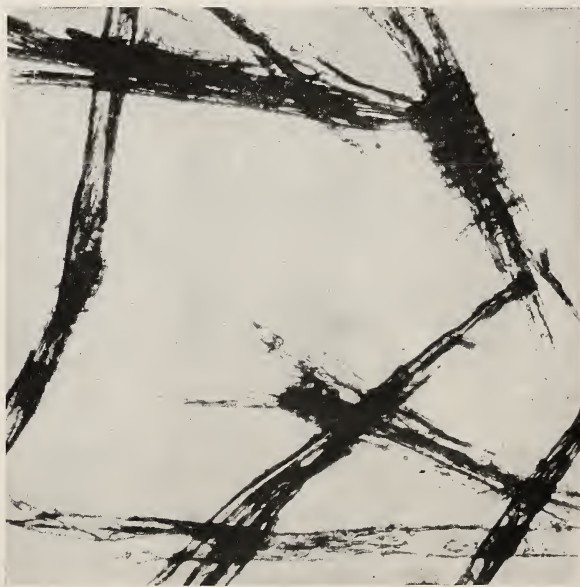
FIG. 18.—Microphotograph of spruce ground wood fiber ( Picea canadensis ). \times 100
