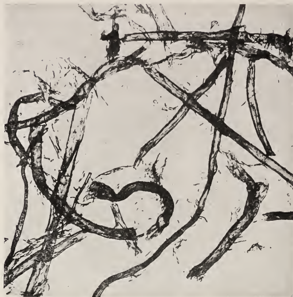
FIG. 17.—Microphotograph of fibers from rag pulp. \times 100
