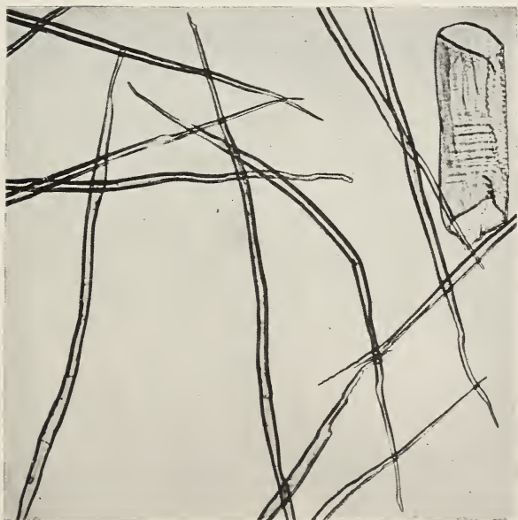
FIG. 16.—Microphotograph of sugar or hard maple fiber ( Acer saccharum ). \times 100
