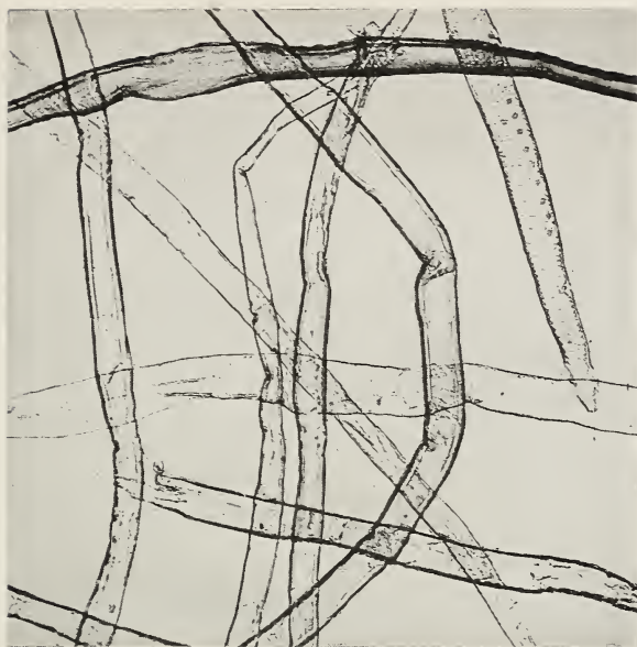
FIG. 15.—Microphotograph of Douglas spruce fiber ( Pseudotsuga taxifolia ). \times 100
