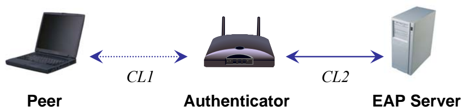
Figure 1: EAP Communication Model
