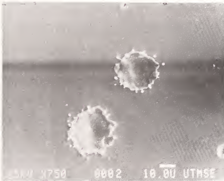
Figure 8. SEM micrograph of damage due to 3 pulses at an average fluence of 0.51 \text{ J/cm}^2 .
