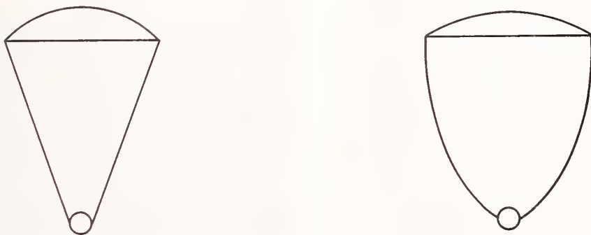
Figure 6 Rotation of the substrate and an oblique vapor incidence results in an increase in the nodule cone angle. The simulation in (b) shows this effect for a nodule without the restrictive influence of the surrounding film. This is typical for the initial stages of nodule growth.
