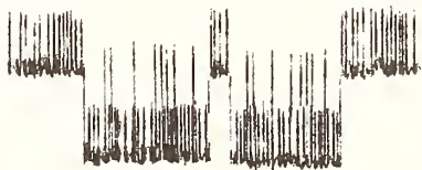
Figure 3a. Burst noise, I_B < 250 nA.
