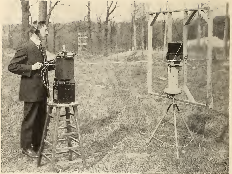
FIG. 23.—Radio direction finder or coil aerial used in measuring the distortion of radio waves in the vicinity of trees, towers, wires, buildings, etc.
