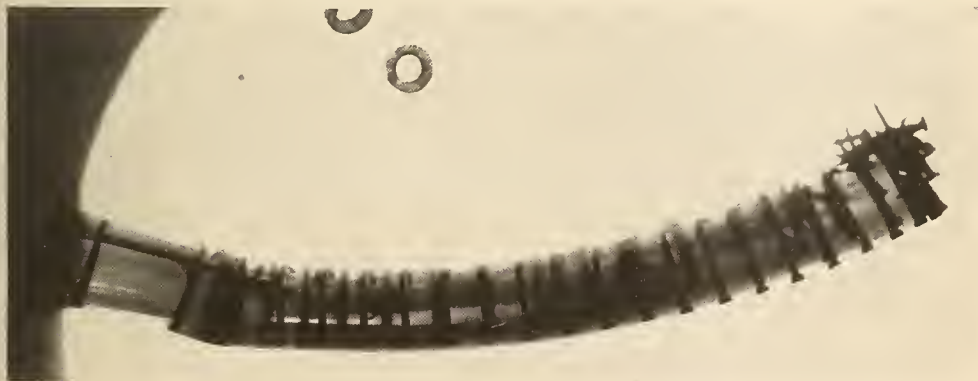
FIG. 34.— Print of radiograph of a repaired shoe
