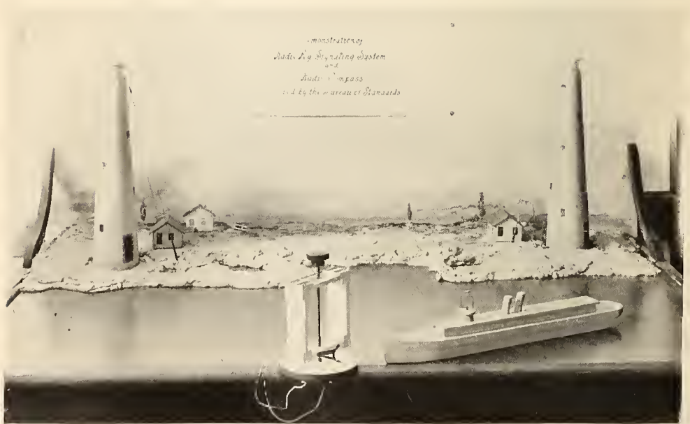
FIG. 24.—Model set-up in the radio laboratory to illustrate the use of the radio direction finder
