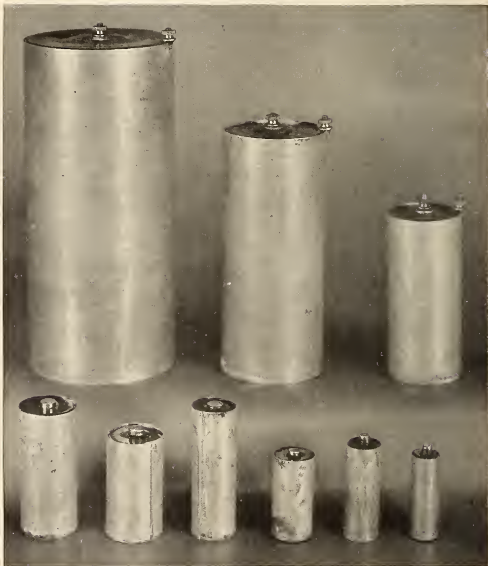
FIG. 10.— The nine sizes of dry cells recommended as standard by the Bureau as the result of its investigations
