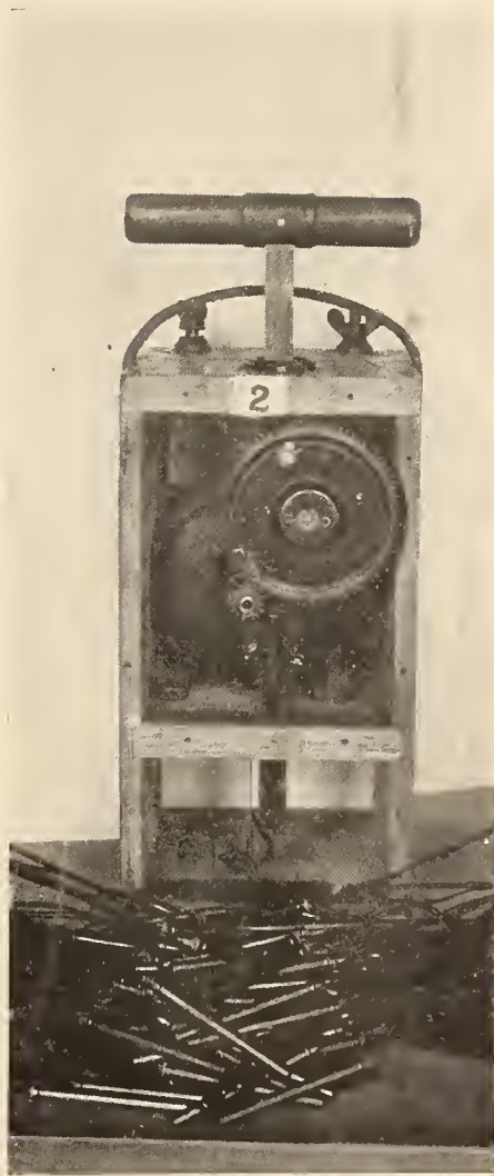
FIG. 12.— The improved blasting machine developed for the use of our overseas forces by the Bureau
