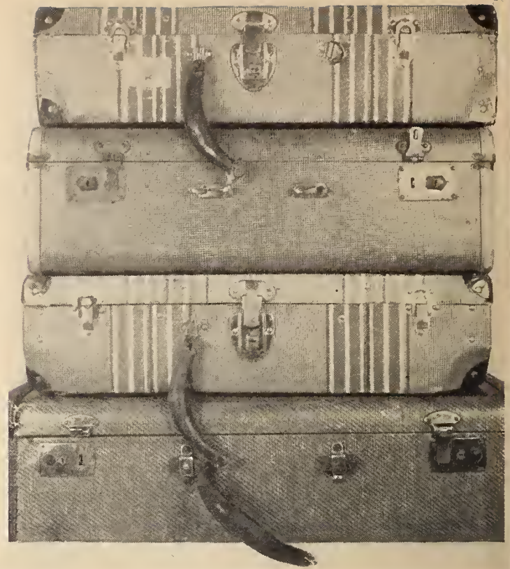
FIGURE 3. Types of damage to luggage handles in service. Top, handle broken away from D-ring, and metal reinforcement in handle pulled out; second, handle disappeared in service; third, rivets fastening handle plate to bag pulled through top of bag; bottom, leather handle broke across slot through which passed metal pin fastening it to bag.
