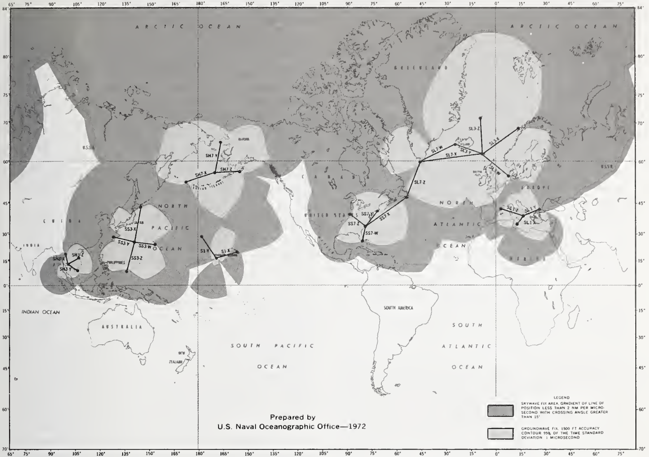
FIGURE 10.18. Coverage of Loran-C navigation system.
