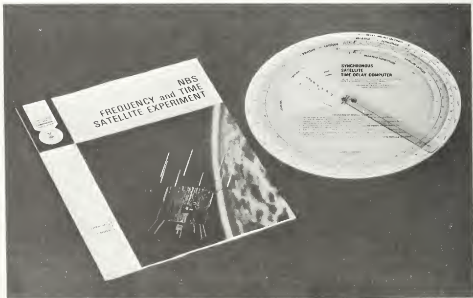
FIGURE 10.46. Slide rule calculator for determining ATS-3 satellite arrival times.
