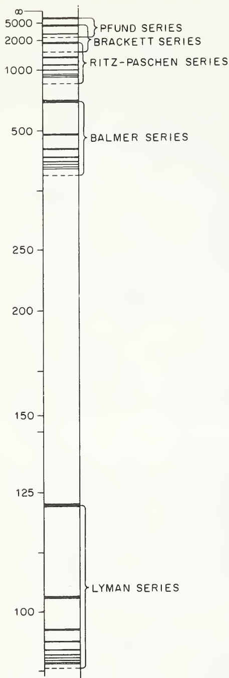
Fig. 3.3. Schematic diagram of the emission spectrum of the hydrogen atom. The intensity of the emission is roughly indicated by the thickness of the lines. The dotted lines are series limits. The wavelength scale is in nanometers. (This figure is a modification of Fig. 8 of Atomic Spectra and Atomic Structure by Gerhard Herzberg, copyright by Dover Publications, 1944.)
