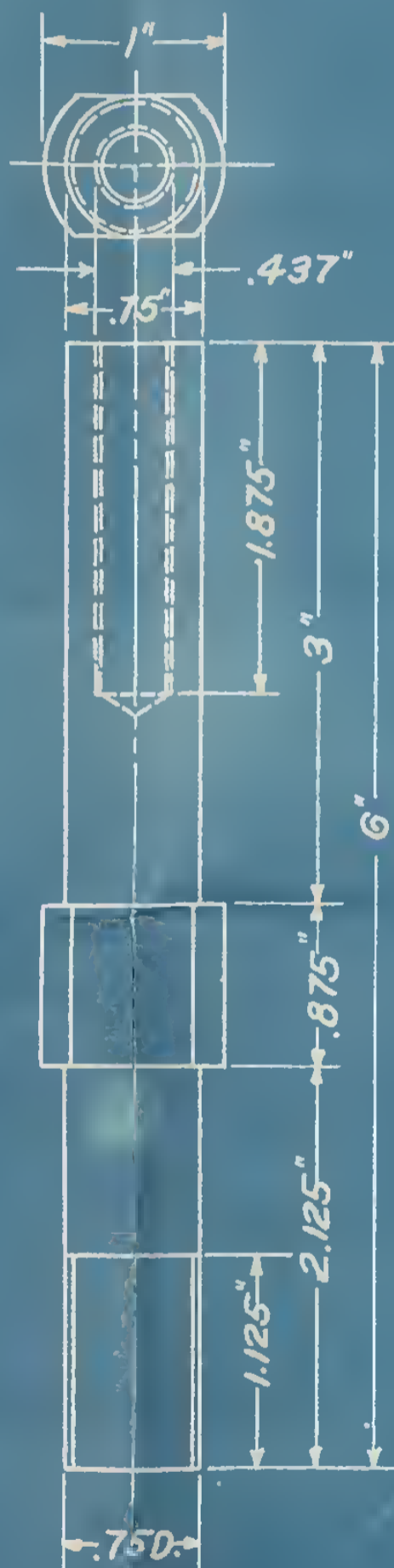
ADAPTER FOR .250" D. SPECIMEN ONE - STEEL
