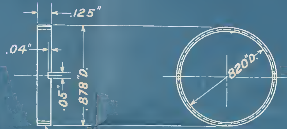
U.S. THREAD 48 PER INCH RETICULE ADJUSTMENT LOCK RING (19) ONE - JAPANNED BRASS
