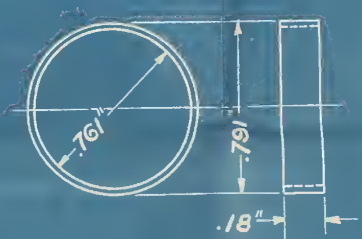
EYEPIECE SPACING RING ONE - JAPANED BRASS
