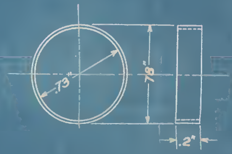
RETICULE SLIP RETAINING RING (21) ONE - JAPANNED BRASS
