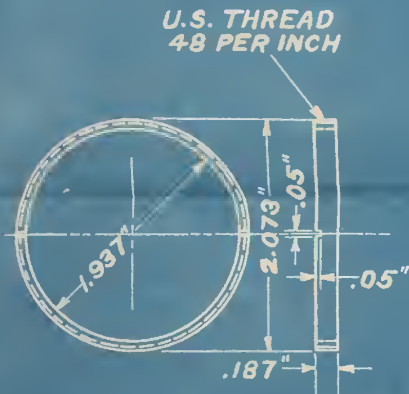
OBJECTIVE LENS (16) SCREW RETAINING RING ONE - JAPANNED BRASS
