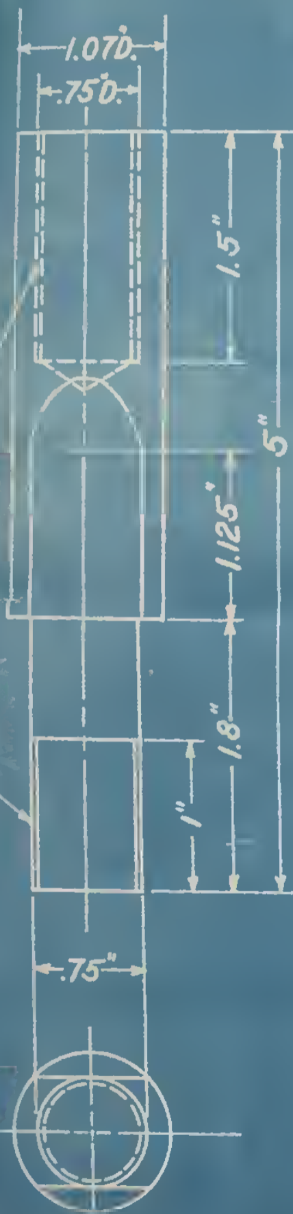
ADAPTER FOR .505" D. SPECIMEN ONE - STEEL
