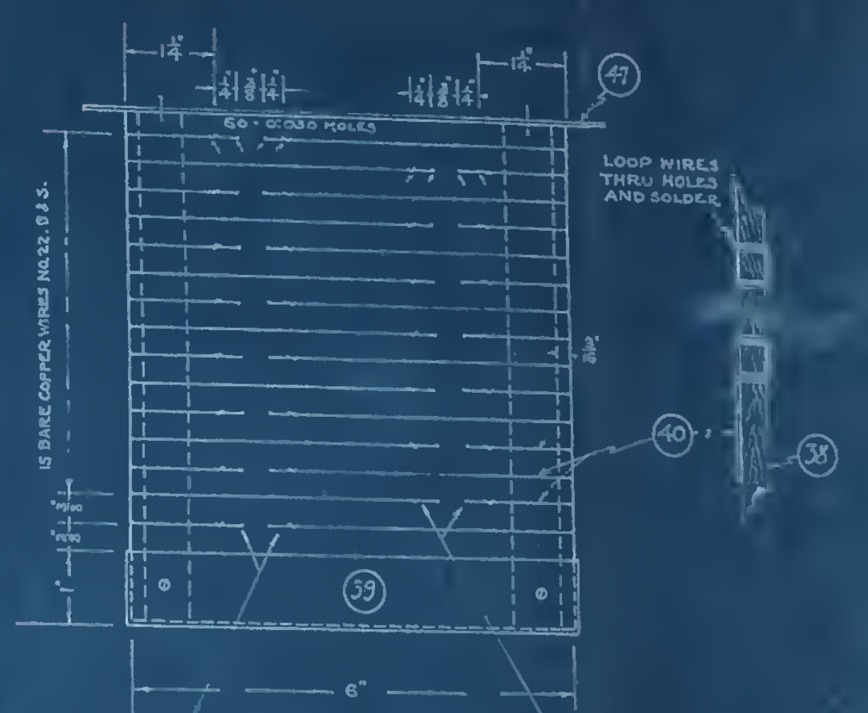
RIGHT END ELEVATION SHOWING ENDS OF WIRE SEWED IN WOOD WITH SOLDERED ENDS
