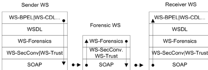
Figure 4. WS-Forensics Stack. Arrows depict how WS-Forensics is applied for a message through web services and their existing stacks.
