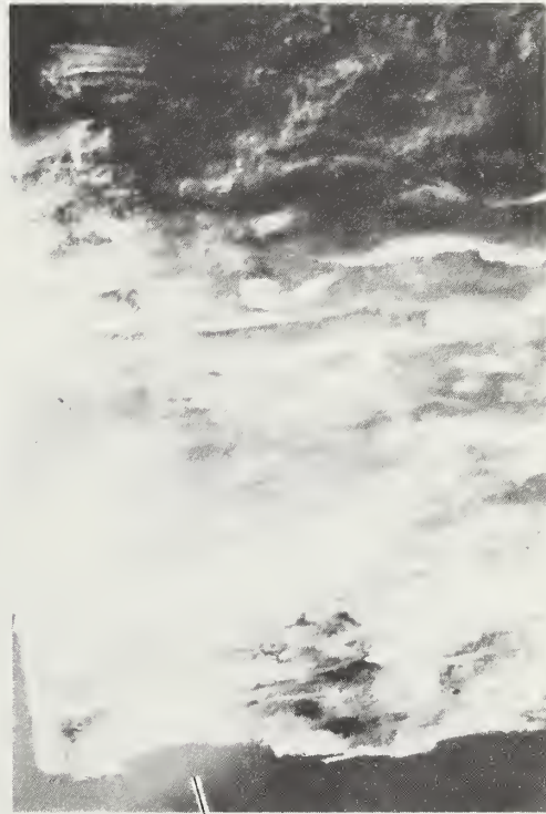
(c) Enlarged view of the fracture surface of another specimen. \sigma_{Cu} = 593.3 Mpa
