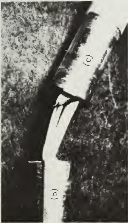
(a) Mixed mode: \sim 55^\circ slant, longitudinal delamination, and bending. Test direction is parallel to axis of end caps. \sigma_{cu} = 854.5 Mpa
