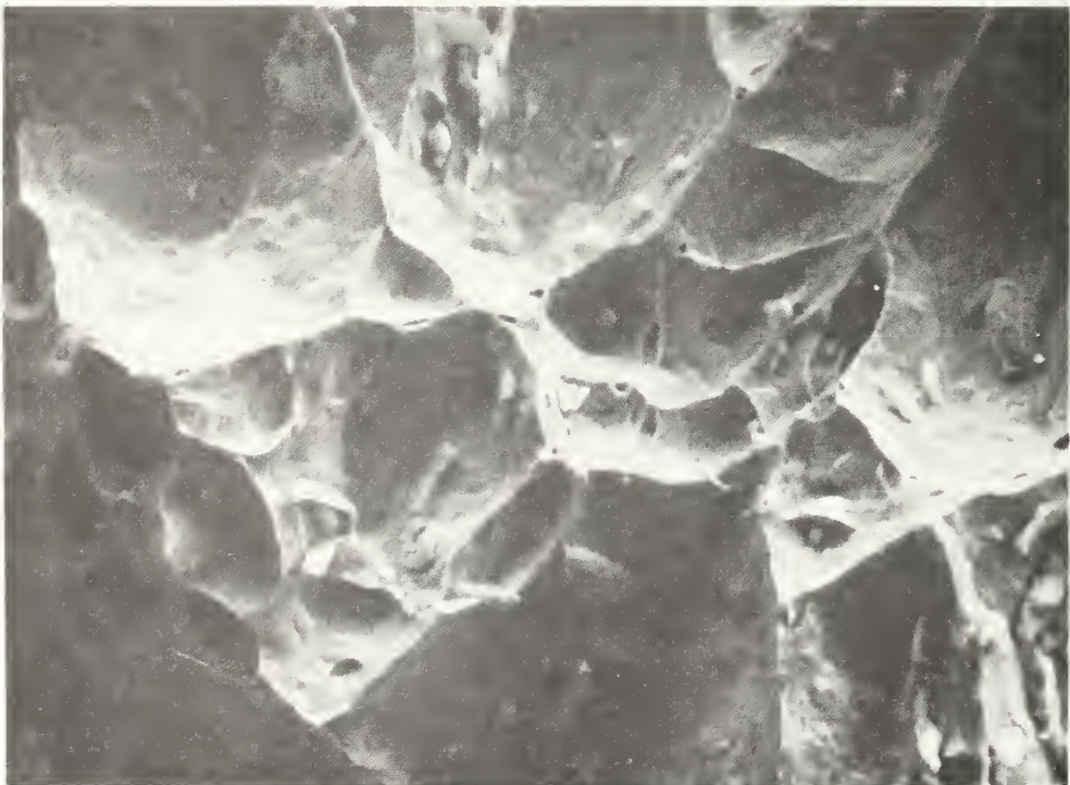
Figure 7. Scanning electron microscopy photograph of Fe-18Cr-10Ni; C+N = 0.325 wt.%. The 4-K fracture surface is shown at 200 X and 1000 X.
