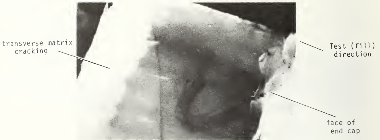
(b) Matrix cracking across specimen gage section face \sigma_{cu} = 561.6 Mpa
