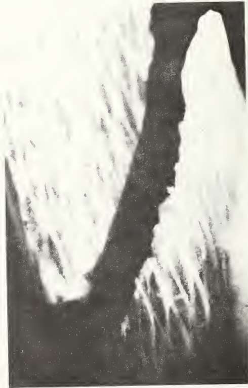
(c) Enlarged view of (a) showing undulating characteristic of the fabric
