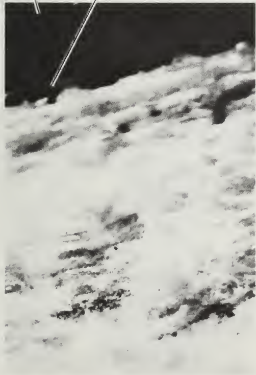
(a) Typical Fracture Surface, Warp Test, 76K. \sigma_{Cu} = 790.4 \text{ Mpa}
