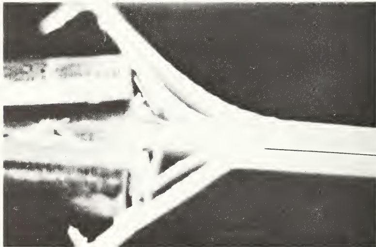
(b) Mixed Mode Failure. No gage section separation. \sigma_{CU} = 849.9 \text{ Mpa}
