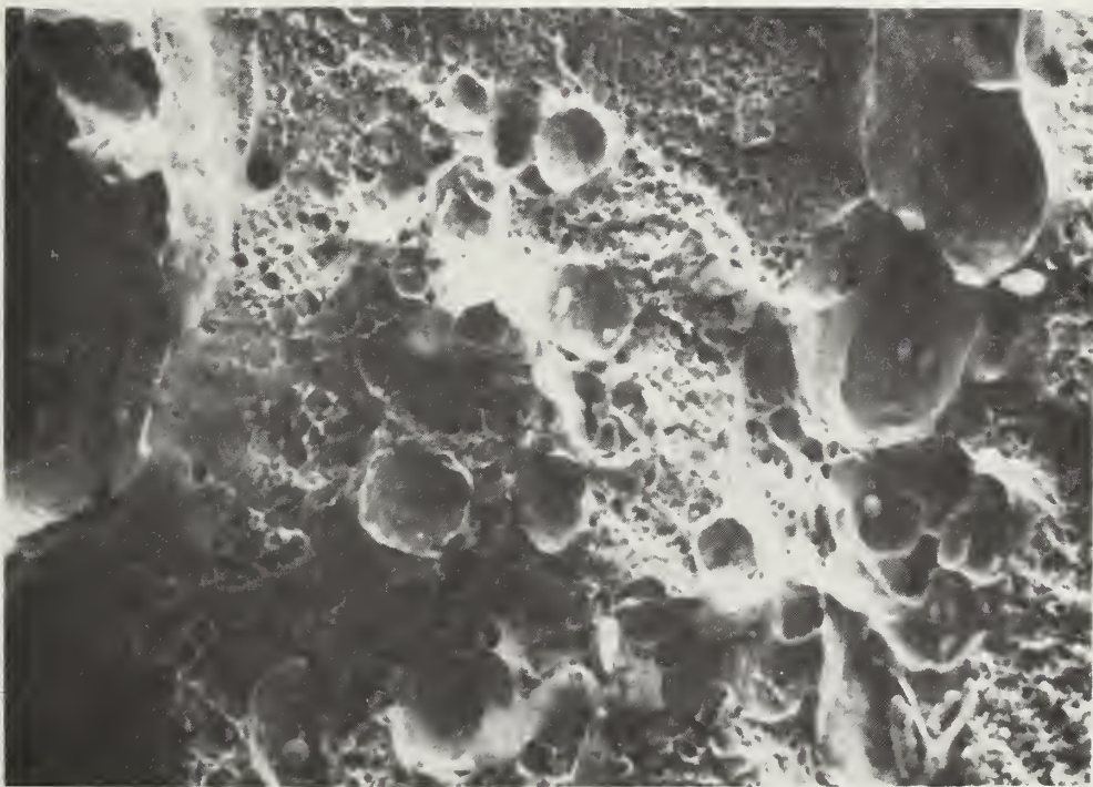
Figure 8. Scanning electron microscopy photograph of Fe-18Cr-10Ni; C+N = 0.067 wt.%. The 4-K fracture surface is shown at 200 X and 1000 X.
