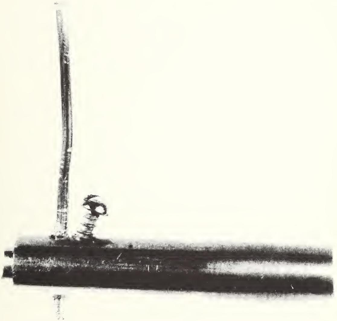
Figure 4 - Experimental connector for wire using a screw wedge.
