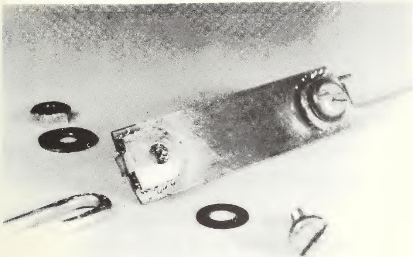
Figure 2 - Experimental connector for aluminum or copper wire designed to be used with Belleville washers so as to compensate for the creep of the wire. The screw does not carry current.
