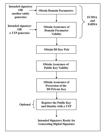
Figure 2: Initial Setup by an Intended Signatory
