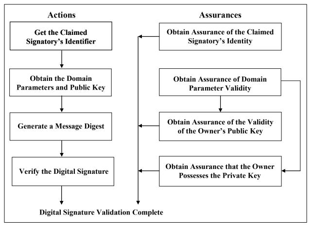
Figure 4: Digital Signature Verification and Validation<sup>6</sup>
